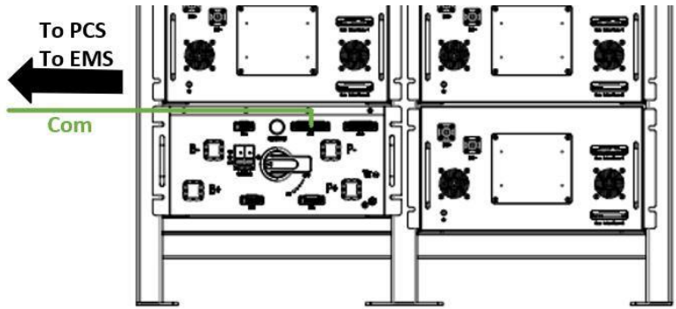
Figure Schematic diagram of battery cluster external communication cable installation
